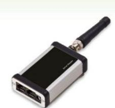
This compact reader is ideally suited for asset tracking, people tracking, and other safety or security applications. It can be used to create RFID networks within buildings. The tag data and reader status information is fed into the end-user application enabling complete management of all tagged assets and the automation of business decisions about them based on accurate and
